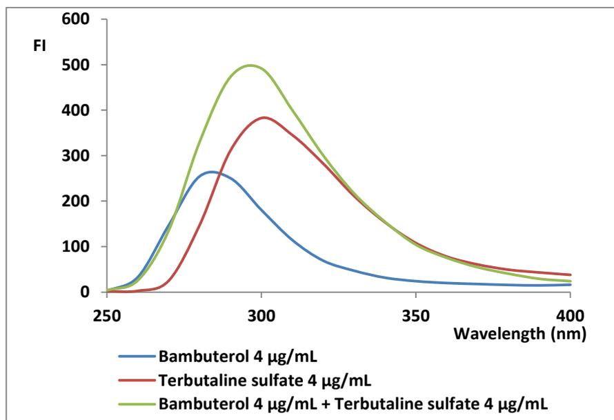
**Figure 2:** Emission spectra of BAM, TER and their combination
