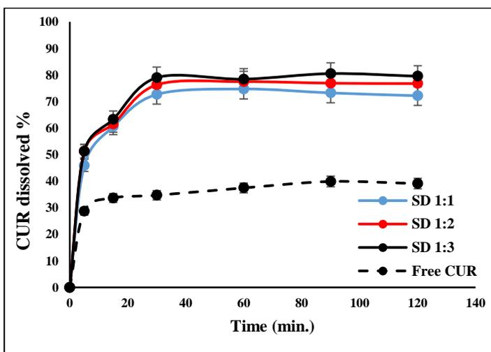
**Figure 10s:** Dissolution profile of CUR from its solid dispersions (SD) with PEG 6000 in phosphate buffer pH 5.5 and 37 °C. Each value represent the mean  $\pm$ SD (n=3).
