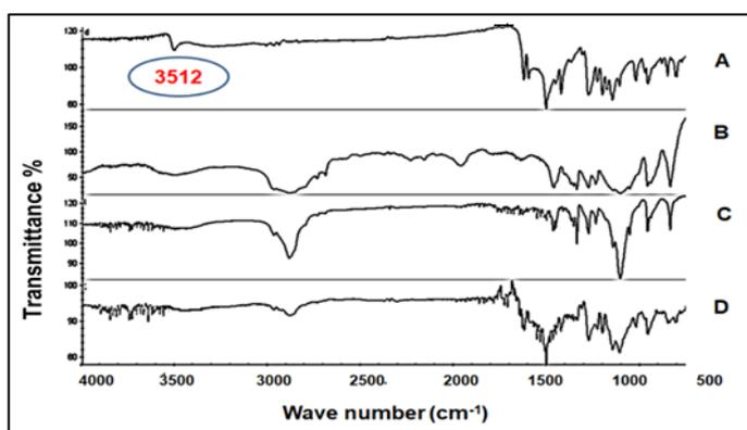
**Figure 6s:** FT- IR spectra of CUR (A), PluF-127 (B), their physical mixture (C) and freeze dried solid dispersion (D) of CUR and PluF-127 at ratio of 1:1.
