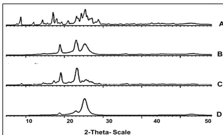
**Figure 7s:** XRD spectra of CUR (A), PluF-127 (B), their physical mixture (C) and freeze dried solid dispersion (D) at ratio 1:1.
