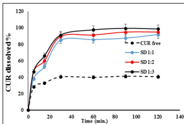
**Figure 6:** Dissolution profile of CUR from its solid dispersions (SD) at different ratios with PVPK30 in phosphate buffer pH 5.5 and 37 °C. Each value represent the mean  $\pm$ SD (n=3).
