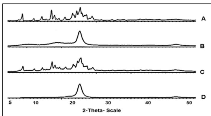
**Figure 3:** XRD spectra of CUR (A), HP $\beta$ -CD (B), their physical mixture (C) and freeze dried solid dispersion (D) at ratio 1:1.
