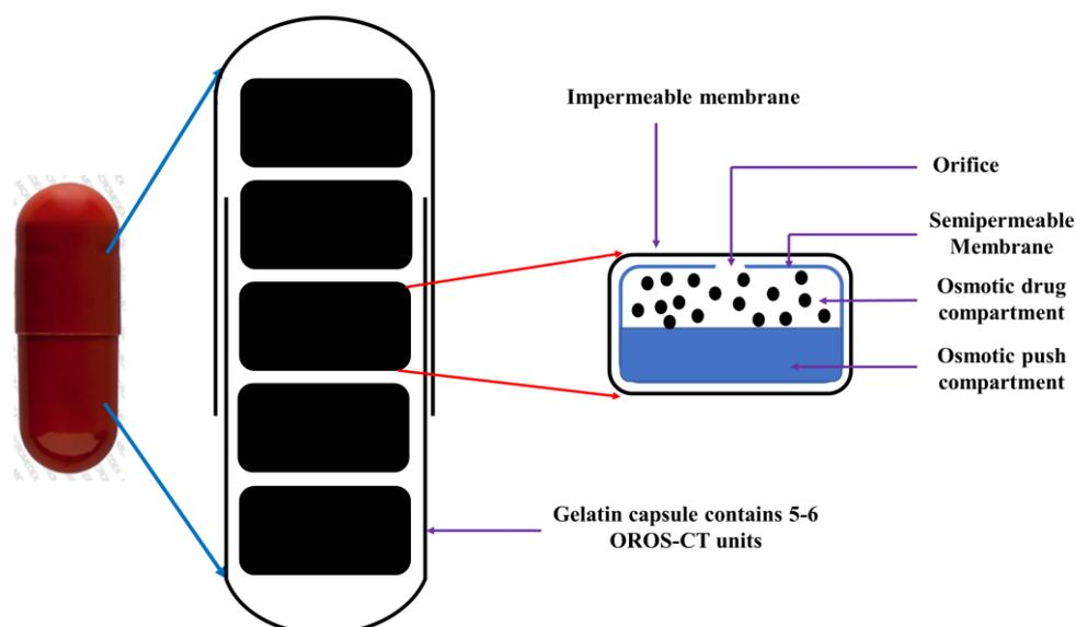
**Figure 4:** Schematic diagram of OROS-CT drug delivery system.
